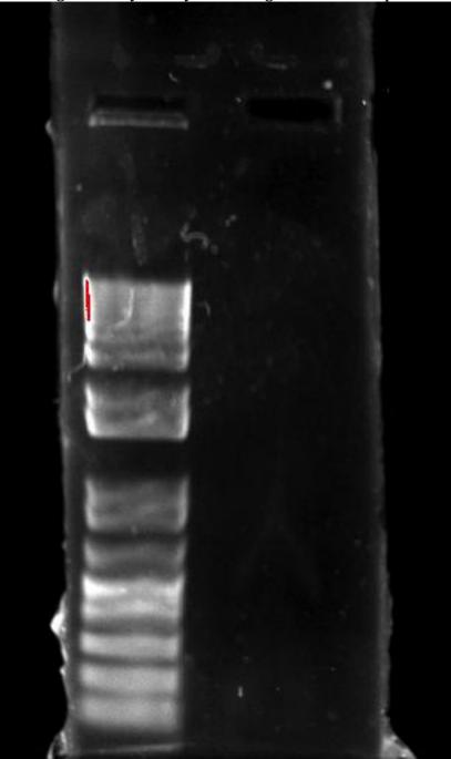
Analysis: lack of clear band at 600bp indicates insufficient amount of insert. Also, these instructions might have been incorrect:
