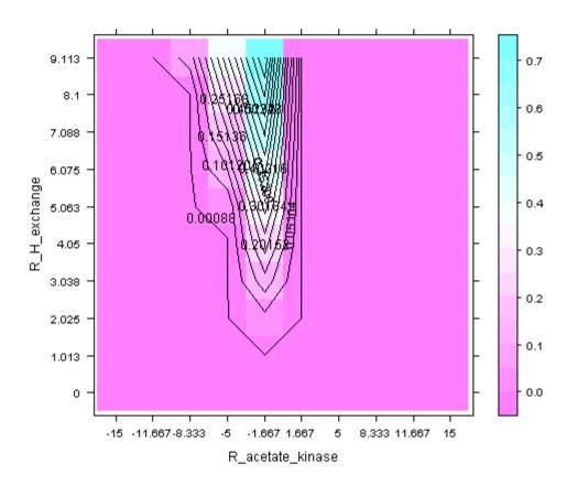
The value marked on the contour represents the flux value of the objective reaction based on the variation of two chosen reactions The color of the graph changes according to the altitude, namely, the objective flux value.
